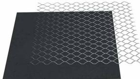
Standard Diamond mesh sheets with Grade D asphalt paper-backed (APB) may be used behind stone, traditional stucco, and tile installations as a code compliant weather resistant barrier. Paper is offset (min) 2" on one long edge on bottom and end, to ensure proper lath-to-lath laps and a minimum 1" paper overhang on the opposing short side. Assure the sheets are shipped-lapped on the wall.
